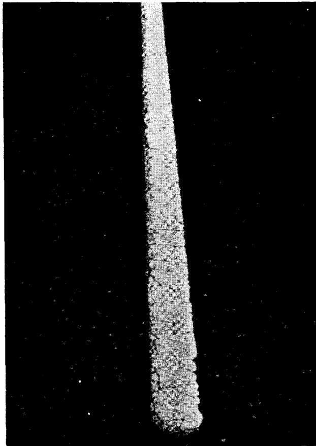
Figure 5. Transverse Cracking of Thermoplastic Material
